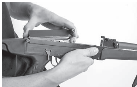
Fig. 29 Taking out the bolt
