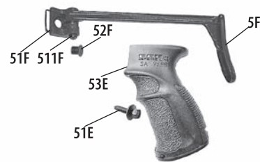
Fig. 19b Metal folding stock with grip 5F - Folding stock, 51F - Suspension of the folding stock, 511F - hinge of the folding stock, 52F - Folding stock scre, 53E - Ergonomic grip, 531E - Ergonomic grip screw
