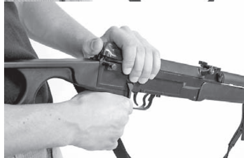
Fig. 28 Removing the return mechanism
